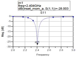
Fig.7 Return loss of Proposed Microstrip patch antenna
