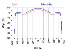
Fig.9 Gain and Directivity of Proposed Microstrip antenna
