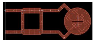
Fig.5 Proposed Antenna Layout design in ADS2009
