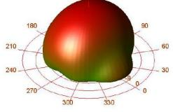
Fig.8 3D Radiation Pattern of Patch Antenna
