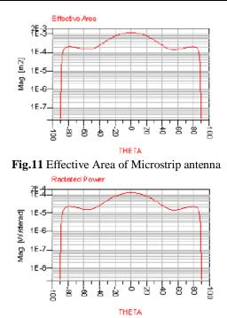
Fig.12 Radiated power of Microstrip antenna
