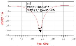
Fig.4 Return loss for Hybrid coupler
